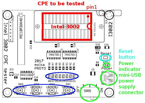
Input buttons & output LEDs Power switch
